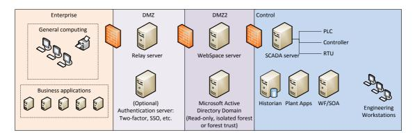
The figure above shows a reference deployment of iFIX components. The control system network is segregated from other untrusted networks such as the enterprise network (also referred to as the business network, corporate network, or intranet) and the internet. Process control network data and applications are authenticated and are exposed in a limited fashion using web-based applications and reporting capabilities.
